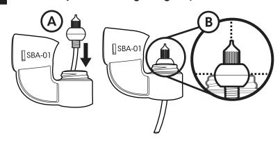
(5) Screw on the cap to lock the nozzle in place.
