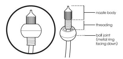
(A) Insert the ball joint back into the siphon adaptor. (B) Make sure that the nozzle and ball joint are sitting straight up.
