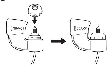
(A) Attach the adaptor onto the eBrush & add the appropriate bottle or siphon cup filled with liquid. (B) Use the center line of the eBrush to confirm that the nozzle is aligned with the eBrush tip.
