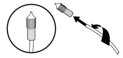
Screw the nozzle back into the ball joint (metal ring facing down) until the nozzle stops.
